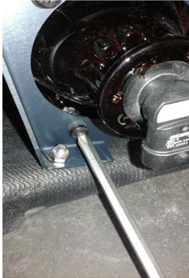
When you are happy with the light adjustment, re-attach the fairing and use the washers and Nylock nuts to secure the bottom of the fairing. Place a black plastic washer under the bolt heads on the fairing side at the top where the fairing bolts to the dashboard. Tighten the Nylock nuts at the base of the fairing.
