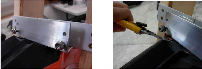
When you have the fender and bracket sitting together, place 2 aluminum washers as spacers on the back bolts ( to level the fender) and tighten all 4 bolts.
