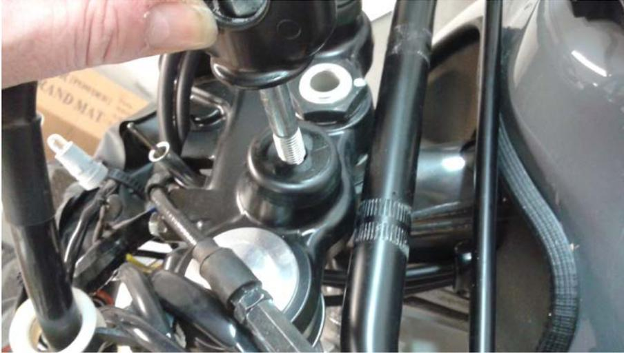
Fit the dashboard under the Bar risers using the OEM bolts and re tighten
