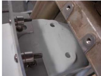
The fender bracket combo will attach to the bottom triple clamp using two , 25mm countersunk bolts anchored into the two threaded holes on the front face of the bottom triple, with a 10mm spacer ( see photo ). This allows the bracket to sit 10mm off the front face.
