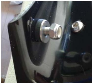
A plastic washer should be fitted under the screw head on the fairing side of the top mount before securing with a flange nut on the dashboard side.
