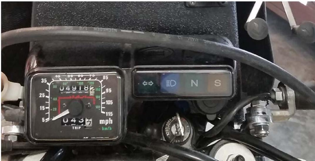
When you are satisfied that the unit is in the right position, mark the position of the mounting holes and the hole for the speedo drive and then remove the dashboard.
