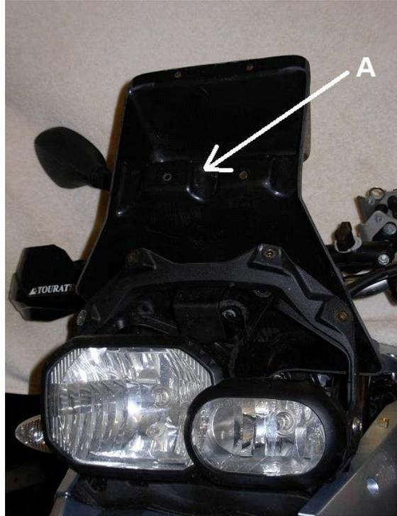
Note that there is a channel molded into the centre of the dash so that you can run wires from the bike up behind the GPS platform. (see photo A)
