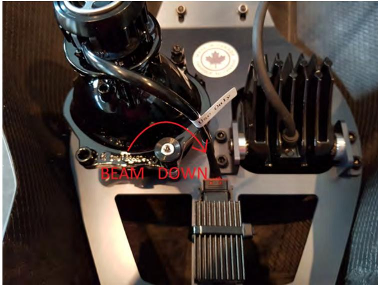
**IMPORTANT :** If your height adjustment causes either lamp to touch the fairing openings it will cause an annoying vibrating noise and excessive wear. In this case, remove fairing and bring the lamp rearwards using the top and bottom adjusters
